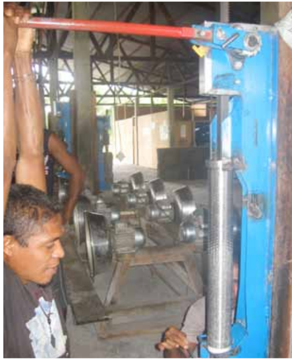
Figure 18. Low pressure oil extraction using a DME press
