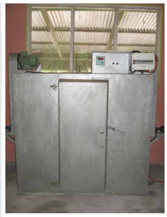
Figure 51. Electrically heated forced draught tray-type dryer at the Food Processing Centre, Kiribati
