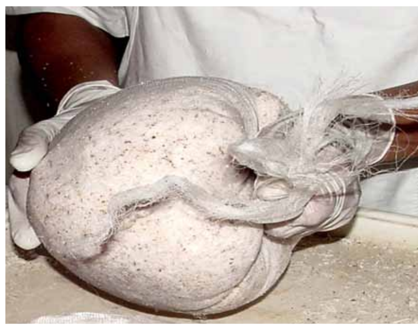
Figure 54. White plastic net bag for grated coconut kernel for extraction in a manually operated milk press
