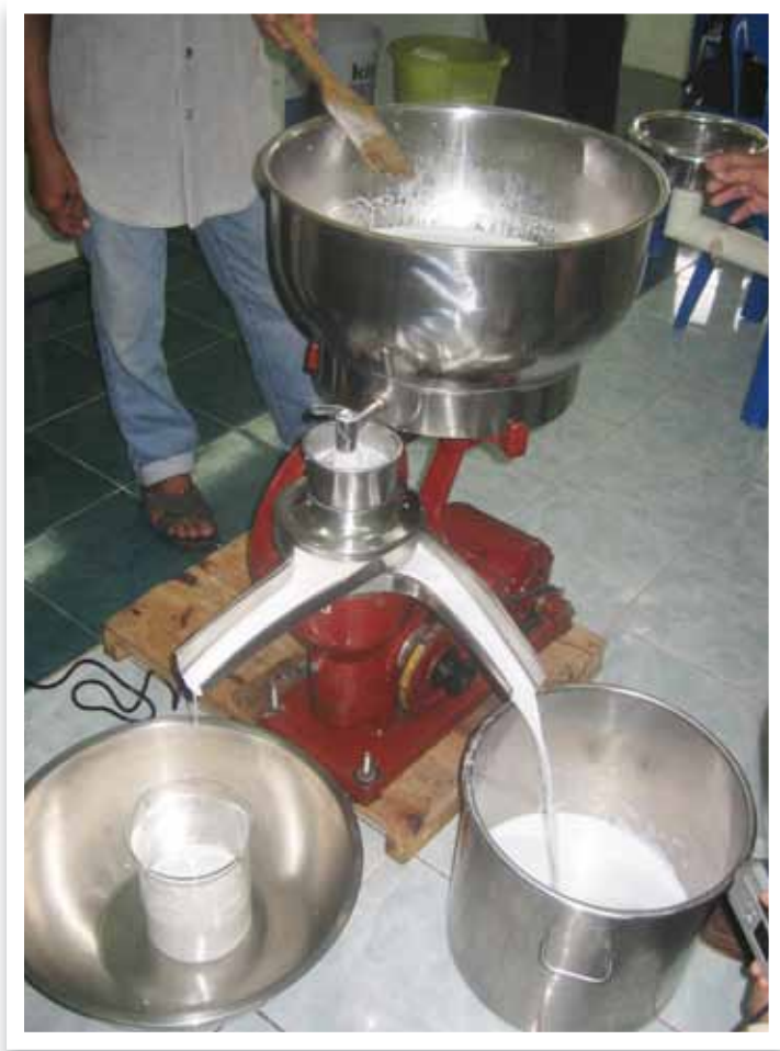
Figure 40. Centrifugal separation of coconut cream and skim milk
