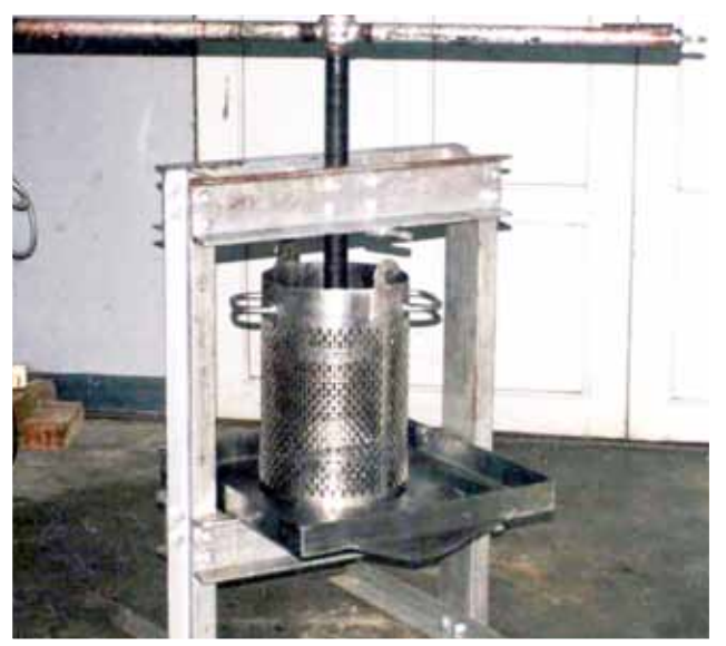
Figure 13. Bridge press developed by the Natural Resources Institute, United Kingdom
