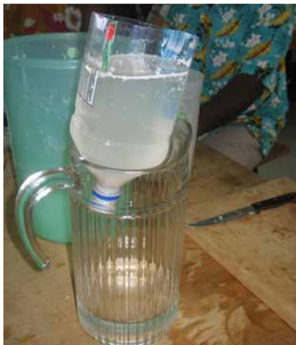
Figure 56. Simple filtration using sterilised cotton balls
