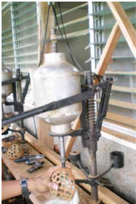
Figure 68. A punching/cutting machine for coconut shell handicrafts
