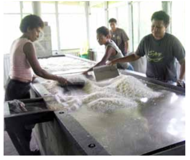
Figure 16. Drying of grated kernel in a standard DME flat bed direct contact type dryer
