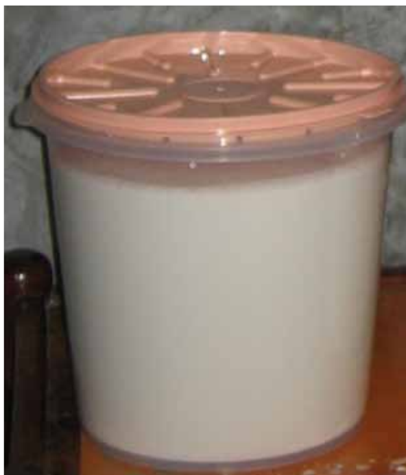
Figure 35. Gravity settling of coconut milk to separate cream and skim milk
