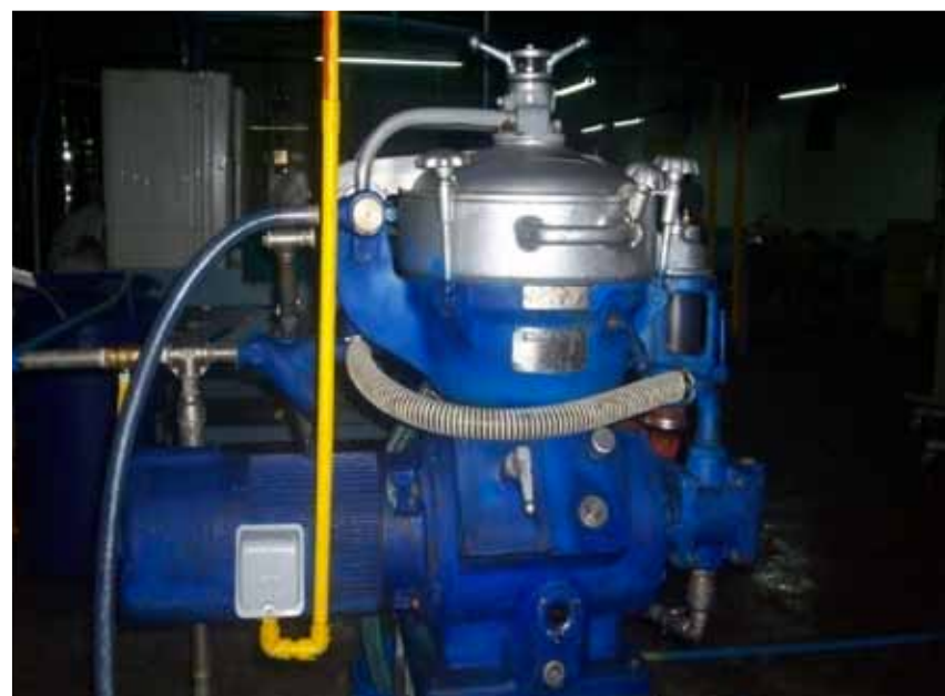
Figure 41. The fresh-wet three-phase centrifuge method
