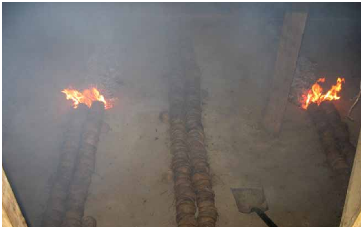
Figure 65. Formation of coconut shell charcoal as fuel in a Sri Lankan copra dryer
