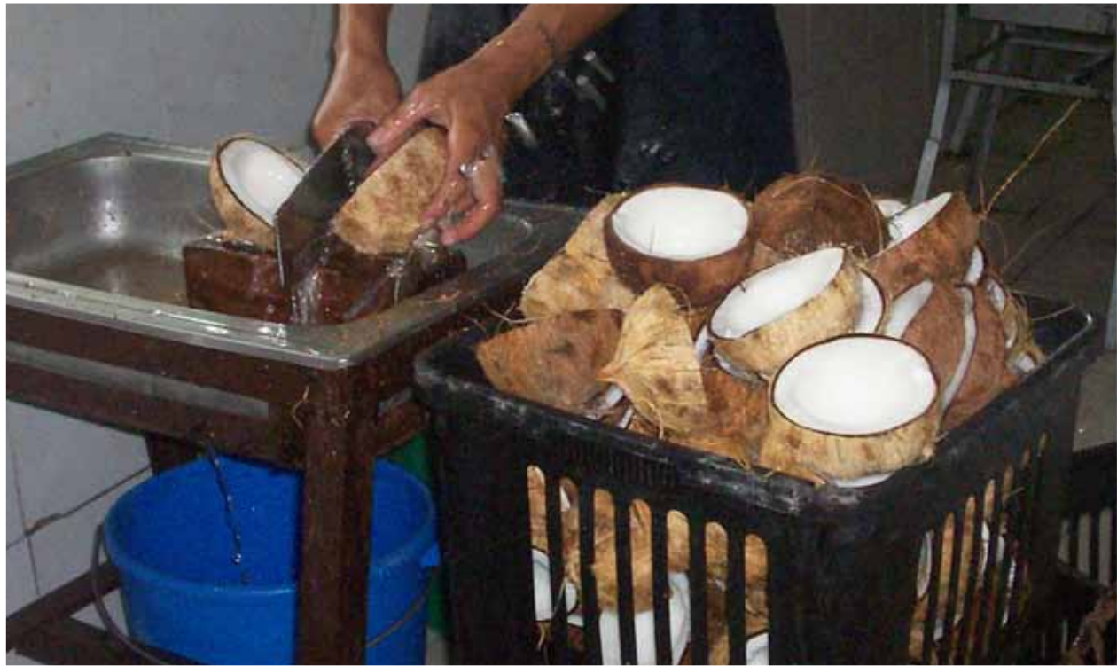
Figure 49. The correct way to split coconuts
