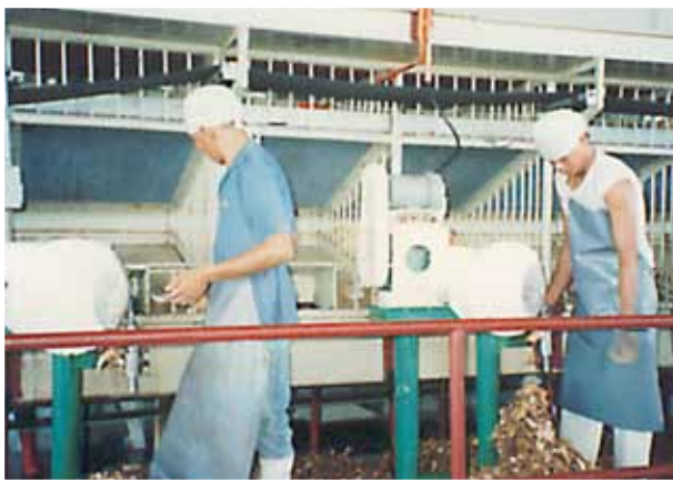
Figure 21. Motorised shelling (left) and manual shelling (right)
