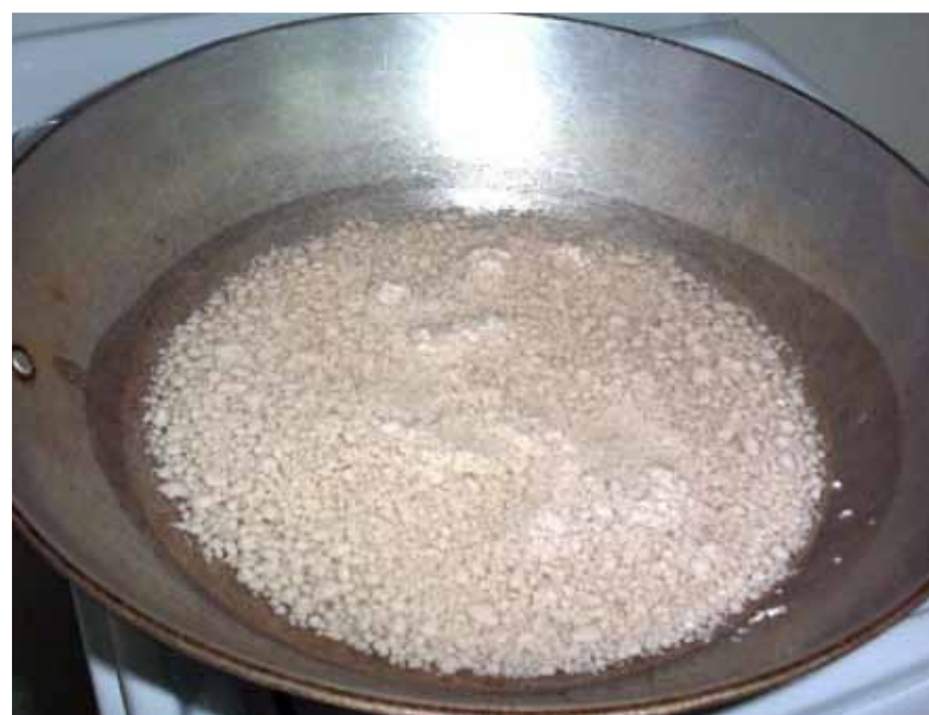
Figure 55. Separation of coconut oil from the coagulated protein (sinusinu) during heating
